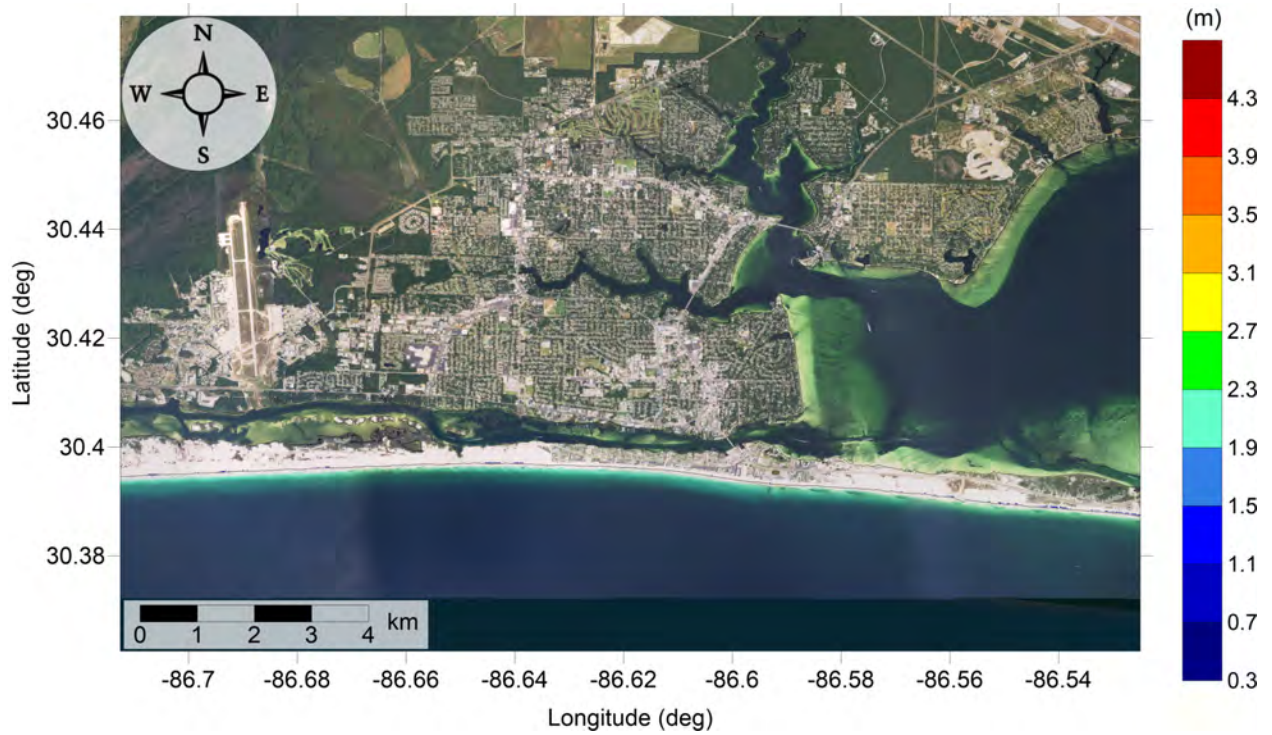
Figure 43: Maximum inundation depth (m) caused by the Probabilistic Submarine Landslide B1 in Okaloosa Island, FL. Contour drawn is the zero-meter contour for land elevation.
