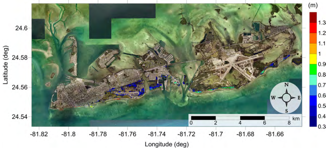
Figure 23: Maximum inundation depth (m) caused by the Probabilistic Submarine Landslide B2 in Key West, FL. Contour drawn is the zero-meter contour for land elevation.
