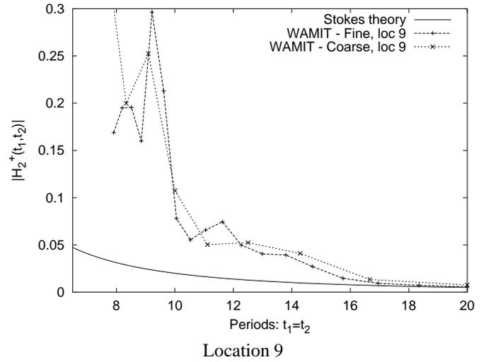
Figure 4: Diagonals of WAMIT Quadratic Transfer Function Matrix
