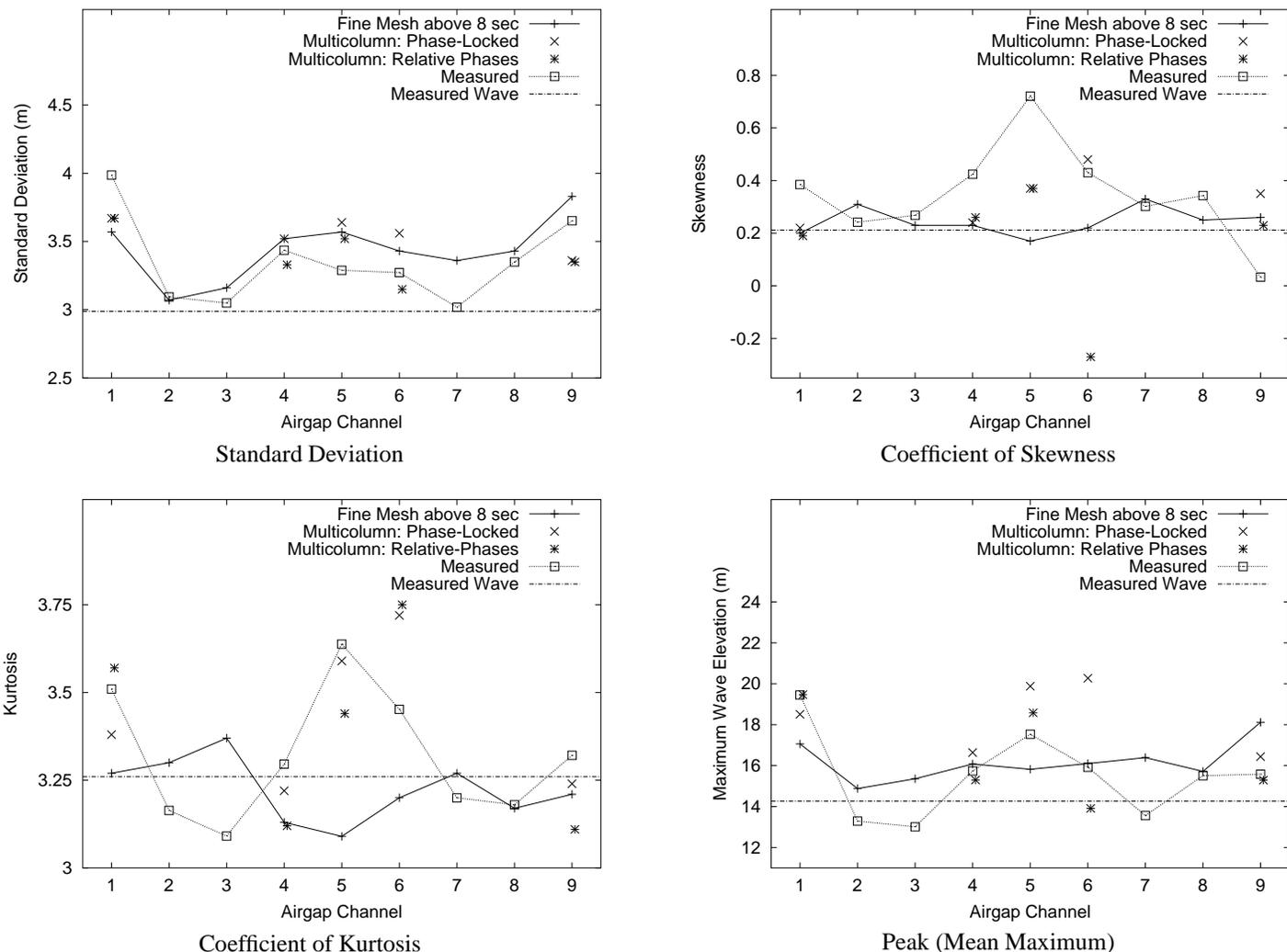
Figure 8: Results based on using WAMIT second-order transfer function results with Stokes second order transfer functions for low periods compared with Multi-column Results  $H_s = 12$  meters,  $T_p = 11.5$  seconds
