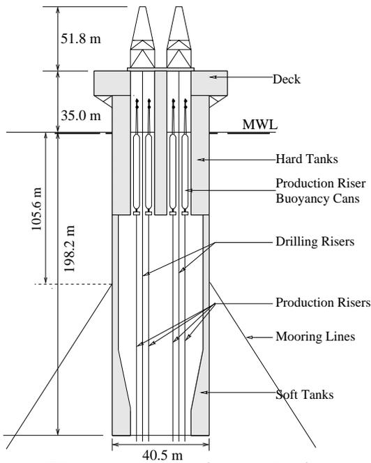
Figure 1: Elevation view of spar platform.
