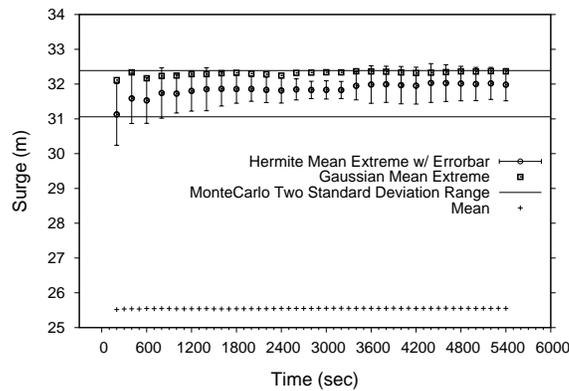
Figure 8: Statistical moments based on short durations used to predict 90 minute maximum. All statistics based on 20 simulations
