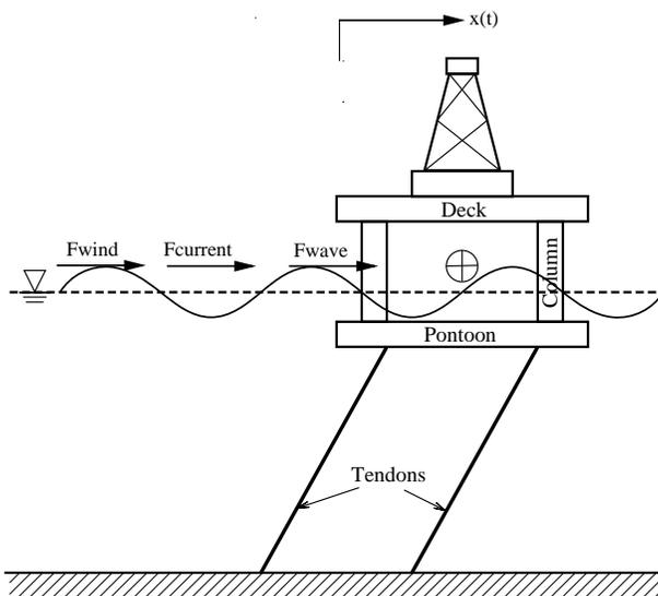
Figure 2: Tension Leg Platform
