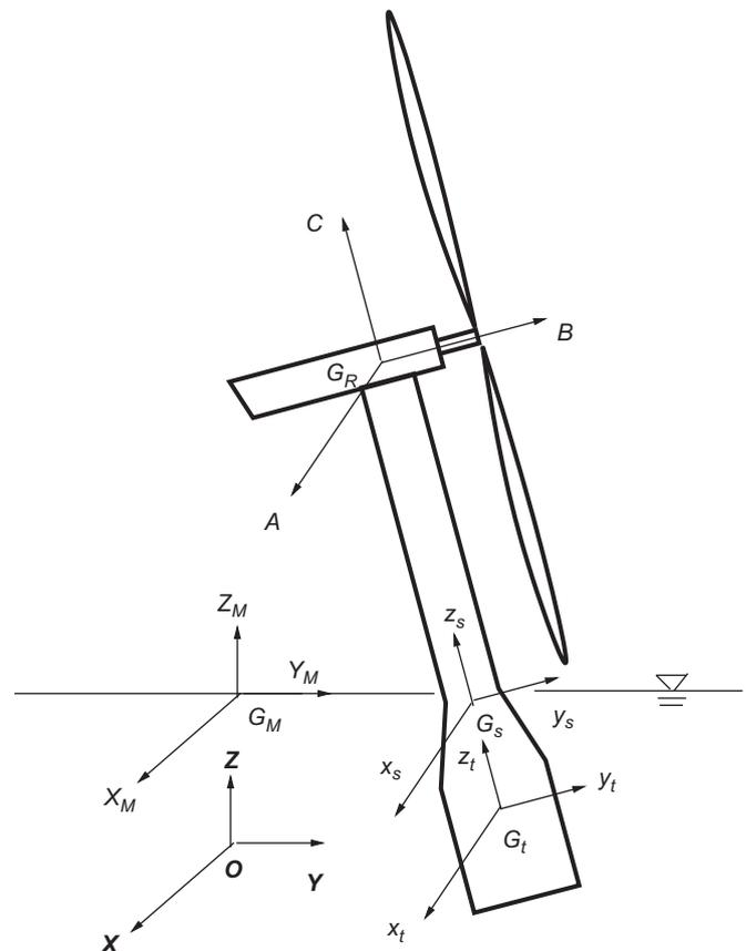
Fig. 1. Coordinate systems used in the application.
