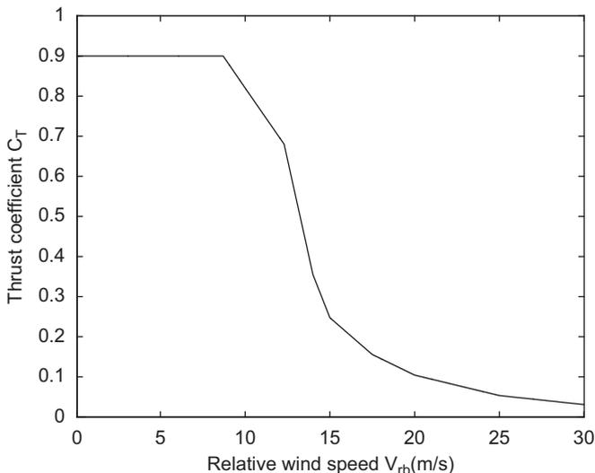
Fig. 3. Thrust force coefficient as a function of relative wind velocity (Nielsen et al., 2006).
