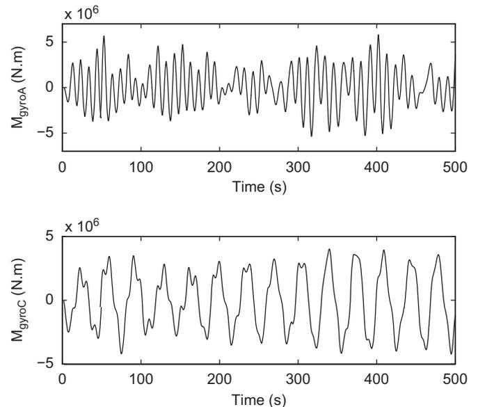
Fig. 12. Gyro moments with nacelle yaw.
