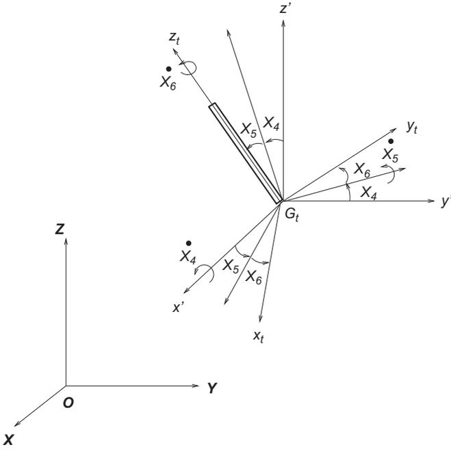
Fig. 2. 1-2-3 sequenced Euler angles in terms of  $X_4$ ,  $X_5$  and  $X_6$ .
