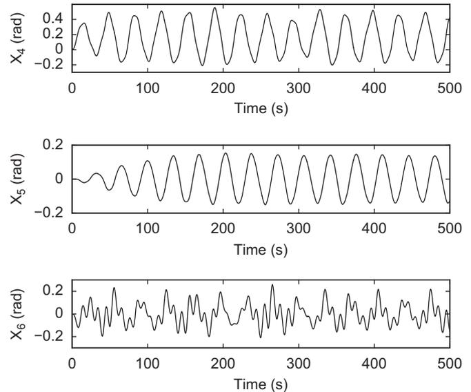
Fig. 8. Rotational motion without nacelle yaw.
