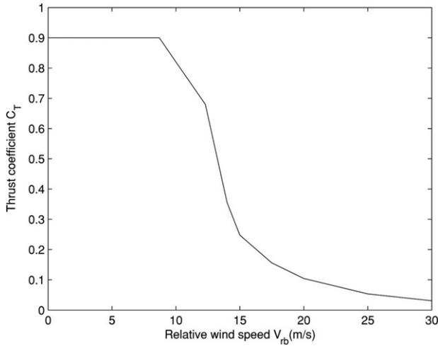
Fig. 3. Thrust coefficient as a function of relative wind velocity [16].
