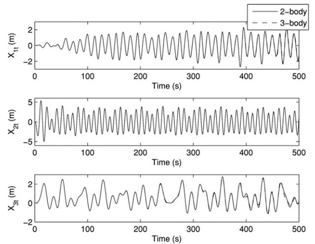
Fig. 9. Translation with variable thrust coefficient: 2-body vs 3-body models.
