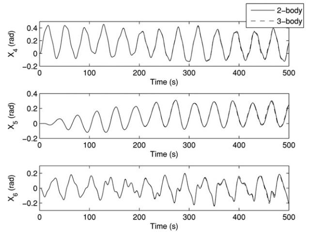
Fig. 8. Rotation with variable thrust coefficient: 2-body vs 3-body models.
