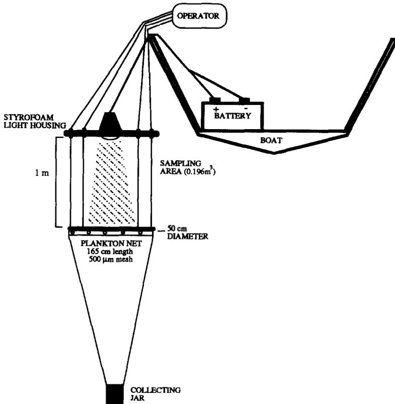
Fig. 1. Schematic representation of the nightlight lift-net.
