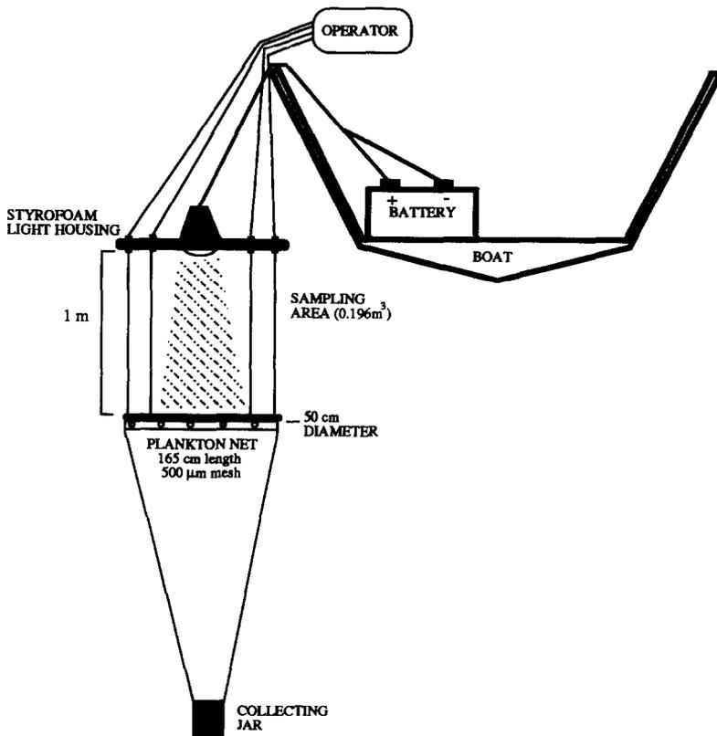
Fig. 1. Schematic representation of the nightlight lift-net.
