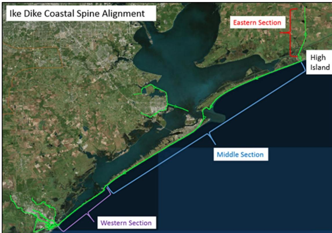
**Figure 2-1.** Schematic of the footprint for the Ike Dike coastal spine concept.
