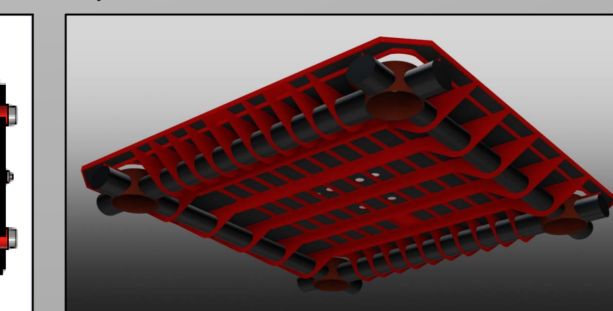
Figure 11. Heave Plate Stiffener Arrangement
